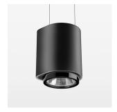
Suspended luminaire with LED, rated life of the LED L80/B10 50000 h (tambient 25°C), colour rendering index CRI > 82, chromaticity tolerance 2 SDCM (initial), reflector with oval light distribution pattern, 3D silicone lens to reduce the proportion of scattered light, reflector pure aluminium 99,99% in MIRO-Silver®, segmented, exchangeable reflector unit in high-sheen black plastic, with glass cover, luminaire housing die-cast aluminium, powdercoated, black
