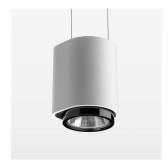
Suspended luminaire with LED, rated life of the LED L80/B10 50000 h (tambient 25°C), colour rendering index CRI > 90, chromaticity tolerance 2 SDCM (initial), reflector with oval light distribution pattern, 3D silicone lens to reduce the proportion of scattered light, reflector pure aluminium 99,99% in MIRO-Silver®, segmented, exchangeable reflector unit in high-sheen black plastic, with glass cover, luminaire housing die-cast aluminium, powdercoated, white
