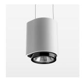
Suspended luminaire with LED, rated life of the LED L80/B10 50000 h (tambient 25°C), colour rendering index CRI > 82, chromaticity tolerance 2 SDCM (initial), reflector with oval light distribution pattern, 3D silicone lens to reduce the proportion of scattered light, reflector pure aluminium 99,99% in MIRO-Silver®, segmented, exchangeable reflector unit in high-sheen black plastic, with glass cover, luminaire housing die-cast aluminium, powdercoated, white
