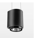
Suspended luminaire with LED, rated life of the LED L80/B10 50000 h (tambient 25°C), colour rendering index CRI > 95, chromaticity tolerance 2 SDCM (initial), reflector with circular light distribution pattern, reflector pure aluminium 99,99% in MIRO-Silver®, segmented and faceted, exchangeable reflector unit in high-sheen black plastic, with glass cover, luminaire housing die-cast aluminium, powder-coated, black Please order canopy and driver unit separatly
