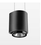
Suspended luminaire with LED, rated life of the LED L80/B10 50000 h (tambient 25°C), colour rendering index CRI > 70, chromaticity tolerance 2 SDCM (initial), reflector with circular light distribution pattern, reflector pure aluminium 99,99% in MIRO-Silver®, segmented and faceted, exchangeable reflector unit in high-sheen black plastic, with glass cover, luminaire housing die-cast aluminium, powder-coated, black Please order canopy and driver unit separatly
