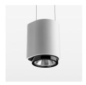
Suspended luminaire with LED, rated life of the LED L80/B10 50000 h (tambient 25°C), colour rendering index CRI > 90, chromaticity tolerance 2 SDCM (initial), reflector with circular light distribution pattern, 3D silicone lens to reduce the proportion of scattered light, reflector pure aluminium 99,99% in MIRO-Silver®, segmented and faceted, exchangeable reflector unit in high-sheen black plastic, with glass cover, luminaire housing die-cast aluminium, powder-coated, white
