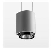
Suspended luminaire with LED, rated life of the LED L80/B10 50000 h (tambient 25°C), colour rendering index CRI > 82, chromaticity tolerance 2 SDCM (initial), reflector with circular light distribution pattern, reflector pure aluminium 99,99% in MIRO-Silver®, segmented and faceted, exchangeable reflector unit in high-sheen black plastic, with glass cover, luminaire housing die-cast aluminium, powder-coated, silver
