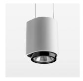
Suspended luminaire with LED, rated life of the LED L80/B10 50000 h (tambient 25°C), colour rendering index CRI > 90, chromaticity tolerance 2 SDCM (initial), reflector with circular light distribution pattern, reflector pure aluminium 99,99% in MIRO-Silver®, segmented and faceted, exchangeable reflector unit in high-sheen black plastic, with glass cover, luminaire housing die-cast aluminium, powder-coated, white Please order canopy and driver unit separatly
