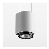
Suspended luminaire with LED, rated life of the LED L80/B10 50000 h (tambient 25°C), colour rendering index CRI > 80, chromaticity tolerance 2 SDCM (initial), reflector with circular light distribution pattern, reflector pure aluminium 99,99% in MIRO-Silver®, segmented and faceted, exchangeable reflector unit in high-sheen black plastic, with glass cover, luminaire housing die-cast aluminium, powder-coated, white Please order canopy and driver unit separatly
