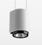
Suspended luminaire with LED, rated life of the LED L80/B10 50000 h (tambient 25°C), colour rendering index CRI > 90, chromaticity tolerance 2 SDCM (initial), reflector with oval light distribution pattern, 3D silicone lens to reduce the proportion of scattered light, reflector pure aluminium 99,99% in MIRO-Silver®, segmented, exchangeable reflector unit in high-sheen black plastic, with glass cover, luminaire housing die-cast aluminium, powder-coated, white
