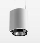
Suspended luminaire with LED, rated life of the LED L80/B10 50000 h (tambient 25°C), colour rendering index CRI > 70, chromaticity tolerance 2 SDCM (initial), reflector with oval light distribution pattern, 3D silicone lens to reduce the proportion of scattered light, reflector pure aluminium 99,99% in MIRO-Silver®, segmented, exchangeable reflector unit in high-sheen black plastic, with glass cover, luminaire housing die-cast aluminium, powder-coated, white
