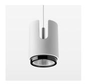
Suspended luminaire with LED, rated life of the LED L80/B10 50000 h (tambient 25°C), colour rendering index CRI > 90, chromaticity tolerance 2 SDCM (initial), reflector with circular light distribution pattern, reflector pure aluminium 99,99% in MIRO-Silver®, segmented and faceted, exchangeable reflector unit in high-sheen black plastic, with glass cover, luminaire housing die-cast aluminium, powder-coated, white
