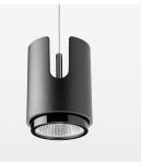
Suspended luminaire with LED, rated life of the LED L80/B10 50000 h (tambient 25°C), colour rendering index CRI > 80, chromaticity tolerance 2 SDCM (initial), reflector with circular light distribution pattern, reflector pure aluminium 99,99% in MIRO-Silver®, segmented and faceted, exchangeable reflector unit in high-sheen black plastic, with glass cover, luminaire housing die-cast aluminium, powder-coated, black Please order canopy and driver unit separatly
