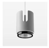
Suspended luminaire with LED, rated life of the LED L80/B10 50000 h (tambient 25°C), colour rendering index CRI > 90, chromaticity tolerance 2 SDCM (initial), reflector with circular light distribution pattern, 3D silicone lens to reduce the proportion of scattered light, reflector pure aluminium 99,99% in MIRO-Silver®, segmented and faceted, exchangeable reflector unit in high-sheen black plastic, with glass cover, luminaire housing die-cast aluminium, powder-coated, silver
