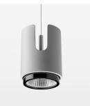
Suspended luminaire with LED, rated life of the LED L80/B10 50000 h (tambient 25°C), colour rendering index CRI > 96, chromaticity tolerance 2 SDCM (initial), reflector with oval light distribution pattern, 3D silicone lens to reduce the proportion of scattered light, reflector pure aluminium 99,99% in MIRO-Silver®, segmented, exchangeable reflector unit in high-sheen black plastic, with glass cover, luminaire housing die-cast aluminium, powder-coated, silver
