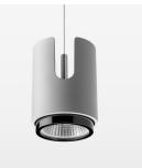
Suspended luminaire with LED, rated life of the LED L80/B10 50000 h (tambient 25°C), colour rendering index CRI > 80, chromaticity tolerance 2 SDCM (initial), reflector with oval light distribution pattern, 3D silicone lens to reduce the proportion of scattered light, reflector pure aluminium 99,99% in MIRO-Silver®, segmented, exchangeable reflector unit in high-sheen black plastic, with glass cover, luminaire housing die-cast aluminium, powder-coated, silver
