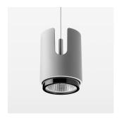
Suspended luminaire with LED, rated life of the LED L80/B10 50000 h (tambient 25°C), colour rendering index CRI > 96, chromaticity tolerance 2 SDCM (initial), reflector with circular light distribution pattern, 3D silicone lens to reduce the proportion of scattered light, reflector pure aluminium 99,99% in MIRO-Silver®, segmented and faceted, exchangeable reflector unit in high-sheen black plastic, with glass cover, luminaire housing die-cast aluminium, powder-coated, silver
