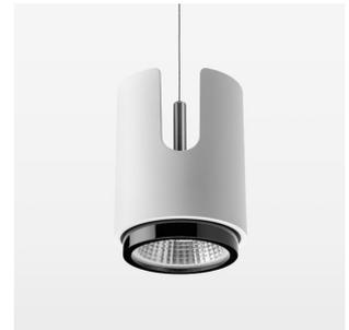
Suspended luminaire with LED, rated life of the LED L80/B10 50000 h (ambient 25°C), colour rendering index CRI > 90, chromaticity tolerance 2 SDCM (initial), reflector with circular light distribution pattern, 3D silicone lens to reduce the proportion of scattered light, reflector pure aluminium 99,99% in MIRO-Silver®, segmented and faceted, exchangeable reflector unit in high-sheen black plastic, with glass cover, luminaire housing die-cast aluminium, powder-coated, white
