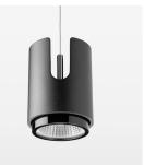
Suspended luminaire with LED, rated life of the LED L80/B10 50000 h (tambient 25°C), colour rendering index CRI > 82, chromaticity tolerance 2 SDCM (initial), reflector with oval light distribution pattern, 3D silicone lens to reduce the proportion of scattered light, reflector pure aluminium 99,99% in MIRO-Silver®, segmented, exchangeable reflector unit in high-sheen black plastic, with glass cover, luminaire housing die-cast aluminium, powder-coated, black
