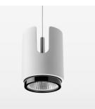
Suspended luminaire with LED, rated life of the LED L80/B10 50000 h (tambient 25°C), colour rendering index CRI > 82, chromaticity tolerance 2 SDCM (initial), reflector with circular light distribution pattern, reflector pure aluminium 99,99% in MIRO-Silver®, segmented and faceted, exchangeable reflector unit in high-sheen black plastic, with glass cover, luminaire housing die-cast aluminium, powder-coated, white Please order canopy and driver unit separatly
