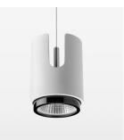
Suspended luminaire with LED, rated life of the LED L80/B10 50000 h (tambient 25°C), colour rendering index CRI > 90, chromaticity tolerance 2 SDCM (initial), reflector with circular light distribution pattern, reflector pure aluminium 99,99% in MIRO-Silver®, segmented and faceted, exchangeable reflector unit in high-sheen black plastic, with glass cover, luminaire housing die-cast aluminium, powder-coated, white Please order canopy and driver unit separatly
