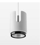
Suspended luminaire with LED, rated life of the LED L80/B10 50000 h (tambient 25°C), colour rendering index CRI > 80, chromaticity tolerance 2 SDCM (initial), reflector with circular light distribution pattern, reflector pure aluminium 99,99% in MIRO-Silver®, segmented and faceted, exchangeable reflector unit in high-sheen black plastic, with glass cover, luminaire housing die-cast aluminium, powder-coated, white Please order canopy and driver unit separatly
