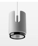
Suspended luminaire with LED, rated life of the LED L80/B10 50000 h (tambient 25°C), colour rendering index CRI > 70, chromaticity tolerance 2 SDCM (initial), reflector with circular light distribution pattern, reflector pure aluminium 99,99% in MIRO-Silver®, segmented and faceted, exchangeable reflector unit in high-sheen black plastic, with glass cover, luminaire housing die-cast aluminium, powder-coated, silver Please order canopy and driver unit separatly
