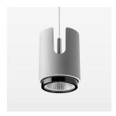
Suspended luminaire with LED, rated life of the LED L80/B10 50000 h (tambient 25°C), colour rendering index CRI > 95, chromaticity tolerance 2 SDCM (initial), reflector with oval light distribution pattern, 3D silicone lens to reduce the proportion of scattered light, reflector pure aluminium 99,99% in MIRO-Silver®, segmented, exchangeable reflector unit in high-sheen black plastic, with glass cover, luminaire housing die-cast aluminium, powdercoated, silver
