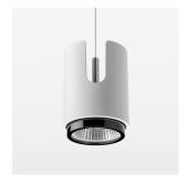
Suspended luminaire with LED, rated life of the LED L80/B10 50000 h (tambient 25°C), colour rendering index CRI > 96, chromaticity tolerance 3 SDCM (initial), reflector with circular light distribution pattern, reflector pure aluminium 99,99% in MIRO-Silver®, segmented and faceted, exchangeable reflector unit in high-sheen black plastic, with glass cover, luminaire housing die-cast aluminium, powder-coated, white
