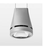
Suspended luminaire with LED, rated life of the LED L80/B10 > 50000 h, colour rendering index CRI > 70, chromaticity tolerance 2 SDCM (initial), reflector with circular light distribution pattern, reflector pure aluminium 99,99% in MIRO-Silver®, luminaire head die-cast aluminium, powder-coated, silver, separate driver unit
