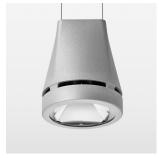
Suspended luminaire with LED, rated life of the LED L80/B10 > 50000 h, colour rendering index CRI > 80, chromaticity tolerance 2 SDCM (initial), reflector with circular light distribution pattern, reflector pure aluminium 99,99% in MIRO-Silver®, luminaire head die-cast aluminium, powder-coated, silver, separate driver unit
