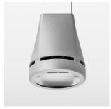
Suspended luminaire with LED, rated life of the LED L80/B10 > 50000 h, colour rendering index CRI > 90, chromaticity tolerance 2 SDCM (initial), reflector with oval light distribution pattern, reflector pure aluminium 99,99% in MIRO-Silver®, luminaire head die-cast aluminium, powder-coated, silver, separate driver unit
