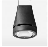
Suspended luminaire with LED, rated life of the LED L80/B10 > 50000 h, colour rendering index CRI > 80, chromaticity tolerance 2 SDCM (initial), reflector with circular light distribution pattern, reflector pure aluminium 99,99% in MIRO-Silver®, luminaire head die-cast aluminium, powder-coated, black
