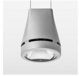
Suspended luminaire with LED, rated life of the LED L80/B10 > 50000 h, colour rendering index CRI > 80, chromaticity tolerance 2 SDCM (initial), reflector with circular light distribution pattern, reflector pure aluminium 99,99% in MIRO-Silver®, luminaire head die-cast aluminium, powder-coated, cilver
