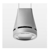
Suspended luminaire with LED, rated life of the LED L80/B10 > 50000 h, colour rendering index CRI > 70, chromaticity tolerance 2 SDCM (initial), reflector with oval light distribution pattern, reflector pure aluminium 99,99% in MIRO-Silver®, luminaire head die-cast aluminium, powder-coated, silver
