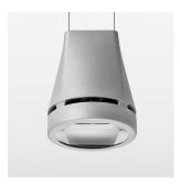
Suspended luminaire with LED, rated life of the LED L80/B10 > 50000 h, colour rendering index CRI > 90, chromaticity tolerance 2 SDCM (initial), reflector with oval light distribution pattern, reflector pure aluminium 99,99% in MIRO-Silver®, luminaire head die-cast aluminium, powder-coated, silver
