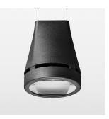
Suspended luminaire with LED, rated life of the LED L80/B10 > 50000 h, colour rendering index CRI > 90, chromaticity tolerance 2 SDCM (initial), reflector with oval light distribution pattern, reflector pure aluminium 99,99% in MIRO-Silver®, luminaire head die-cast aluminium, powder-coated, black
