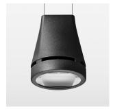
Suspended luminaire with LED, rated life of the LED L80/B10 > 50000 h, colour rendering index CRI > 80, chromaticity tolerance 2 SDCM (initial), reflector with oval light distribution pattern, reflector pure aluminium 99,99% in MIRO-Silver®, luminaire head die-cast aluminium, powder-coated, black
