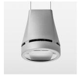
Suspended luminaire with LED, rated life of the LED L80/B10 > 50000 h, colour rendering index CRI > 80, chromaticity tolerance 2 SDCM (initial), reflector with oval light distribution pattern, reflector pure aluminium 99,99% in MIRO-Silver®, luminaire head die-cast aluminium, powder-coated, silver
