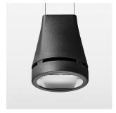
Suspended luminaire with LED, rated life of the LED L80/B10 > 50000 h, colour rendering index CRI > 80, chromaticity tolerance 2 SDCM (initial), reflector with oval light distribution pattern, reflector pure aluminium 99,99% in MIRO-Silver®, luminaire head die-cast aluminium, powder-coated, black
