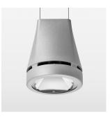
Suspended luminaire with LED, rated life of the LED L80/B10 > 50000 h, colour rendering index CRI > 90, chromaticity tolerance 2 SDCM (initial), reflector with circular light distribution pattern, reflector pure aluminium 99,99% in MIRO-Silver®, luminaire head die-cast aluminium, powder-coated, silver
