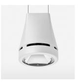
Suspended luminaire with LED, rated life of the LED L80/B10 > 50000 h, colour rendering index CRI > 80, chromaticity tolerance 2 SDCM (initial), reflector with circular light distribution pattern, reflector pure aluminium 99,99% in MIRO-Silver®, luminaire head die-cast aluminium, powder-coated, white
