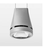
Suspended luminaire with LED, rated life of the LED L80/B10 > 50000 h, colour rendering index CRI > 80, chromaticity tolerance 2 SDCM (initial), reflector with circular light distribution pattern, reflector pure aluminium 99,99% in MIRO-Silver®, luminaire head die-cast aluminium, powder-coated, silver
