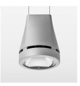
Suspended luminaire with LED, rated life of the LED L80/B10 > 50000 h, colour rendering index CRI > 70, chromaticity tolerance 2 SDCM (initial), reflector with circular light distribution pattern, reflector pure aluminium 99,99% in MIRO-Silver®, luminaire head die-cast aluminium, powder-coated, silver
