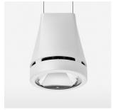
Suspended luminaire with LED, rated life of the LED L80/B10 > 50000 h, colour rendering index CRI > 90, chromaticity tolerance 2 SDCM (initial), reflector with circular light distribution pattern, reflector pure aluminium 99,99% in MIRO-Silver®, luminaire head die-cast aluminium, powder-coated, white
