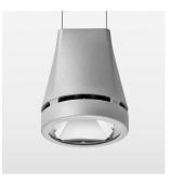
Suspended luminaire with LED, rated life of the LED L80/B10 > 50000 h, colour rendering index CRI > 80, chromaticity tolerance 2 SDCM (initial), reflector with circular light distribution pattern, reflector pure aluminium 99,99% in MIRO-Silver®, luminaire head die-cast aluminium, powder-coated, silver
