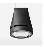
Suspended luminaire with LED, rated life of the LED L80/B10 > 50000 h, colour rendering index CRI > 80, chromaticity tolerance 2 SDCM (initial), reflector with circular light distribution pattern, reflector pure aluminium 99,99% in MIRO-Silver®, canopy sheet steel, powder-coated, luminaire head die-cast aluminium, powder-coated, black
