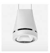
Suspended luminaire with LED, rated life of the LED L80/B10 > 50000 h, colour rendering index CRI > 80, chromaticity tolerance 2 SDCM (initial), reflector with circular light distribution pattern, reflector pure aluminium 99,99% in MIRO-Silver®, canopy sheet steel, powder-coated, luminaire head die-cast aluminium, powder-coated, white
