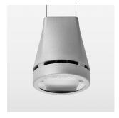
Suspended luminaire with LED, rated life of the LED L80/B10 > 50000 h, colour rendering index CRI > 80, chromaticity tolerance 2 SDCM (initial), reflector with oval light distribution pattern, reflector pure aluminium 99,99% in MIRO-Silver®, canopy sheet steel, powder-coated, luminaire head die-cast aluminium, powder-coated, silver
