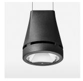
Suspended luminaire with LED, rated life of the LED L80/B10 > 50000 h, colour rendering index CRI > 80, chromaticity tolerance 2 SDCM (initial), reflector with circular light distribution pattern, reflector pure aluminium 99,99% in MIRO-Silver®, luminaire head die-cast aluminium, powder-coated, black, separate driver unit
