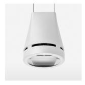
Suspended luminaire with LED, rated life of the LED L80/B10 > 50000 h, colour rendering index CRI > 80, chromaticity tolerance 2 SDCM (initial), reflector with oval light distribution pattern, reflector pure aluminium 99,99% in MIRO-Silver®, canopy sheet steel, powder-coated, luminaire head die-cast aluminium, powder-coated, white
