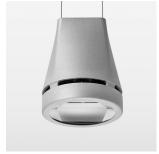
Suspended luminaire with LED, rated life of the LED L80/B10 > 50000 h, colour rendering index CRI > 80, chromaticity tolerance 2 SDCM (initial), reflector with oval light distribution pattern, reflector pure aluminium 99,99% in MIRO-Silver®, luminaire head die-cast aluminium, powder-coated, silver, separate driver unit
