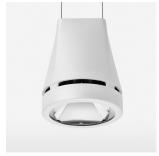
Suspended luminaire with LED, rated life of the LED L80/B10 > 50000 h, colour rendering index CRI > 90, chromaticity tolerance 2 SDCM (initial), reflector with circular light distribution pattern, reflector pure aluminium 99,99% in MIRO-Silver®, canopy sheet steel, powder-coated, luminaire head die-cast aluminium, powder-coated, white
