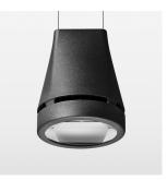
Suspended luminaire with LED, rated life of the LED L80/B10 > 50000 h, colour rendering index CRI > 90, chromaticity tolerance 2 SDCM (initial), reflector with oval light distribution pattern, reflector pure aluminium 99,99% in MIRO-Silver®, luminaire head die-cast aluminium, powder-coated, black, separate driver unit
